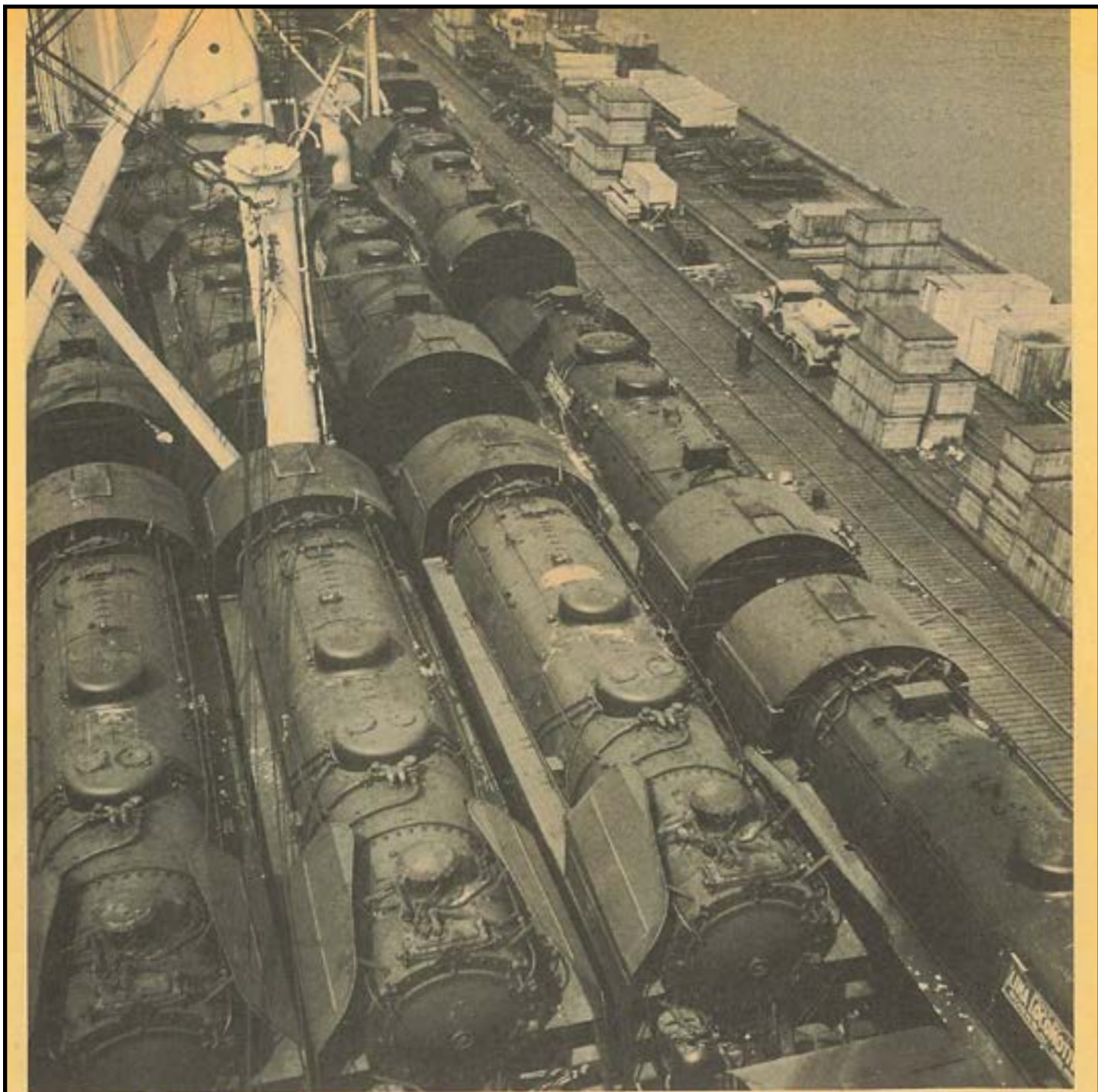
Stacks covered, buffers removed, cabs boarded, a total of 1340 engines and tenders left Weehawken, bound for France. Photograph from Lima Locomotive Works
